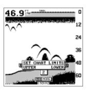
In this example, we're setting the upper limit. Use the up and down arrow keys to select the number, the right and left arrow keys to move to the next number. When the limit shows the desired depth, press the ENT key. The screen shown below appears.
